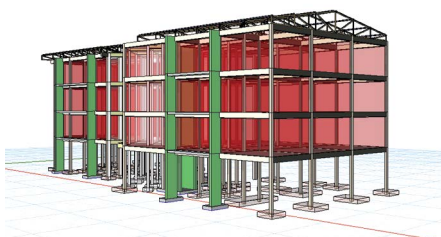
General Medical Laboratory Reinforced Concrete Frames with Shearwalls Total Area: 780 sq. meters
