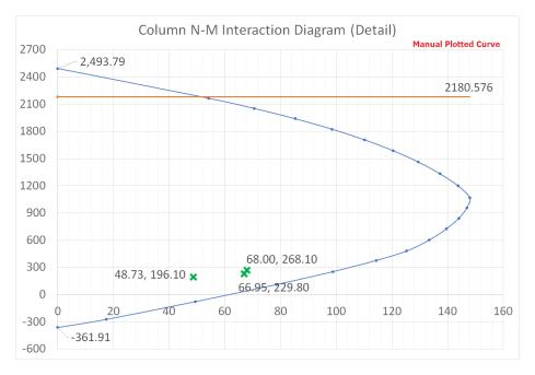
The curve for direction 3 (M22) about "plane X" from ProtaStructure is shown below:
