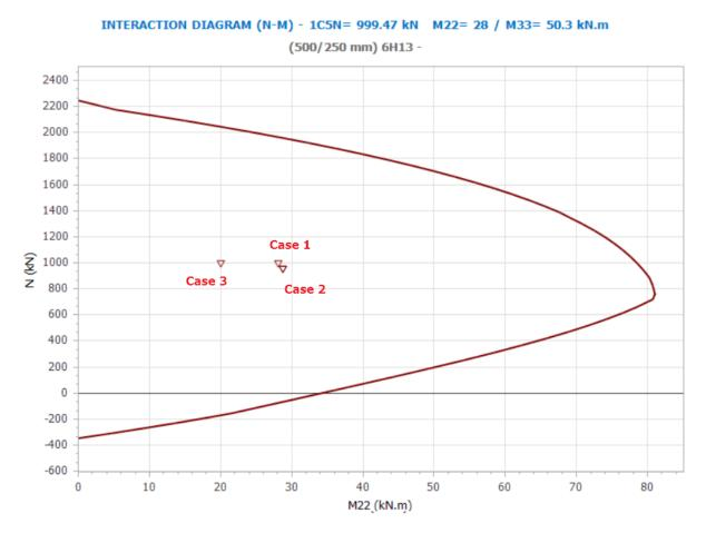
The curve for direction 3 (M22) about "plane X" from ProtaStructure is shown below:
