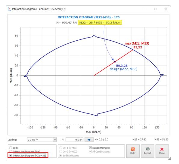
The above is the moment capacity curve expressed in moments in two directions, respectively (M22, M33) for a given axial load. This curve is plotted for the case N = 999.47 kN, obtained for critical load combination 2.
