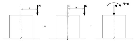
As the eccentricity "e" changes from the section centroid, behaviours of a column/wall and stress distribution in the section will be generated differently. These are used to plot the Axial Load to Moment (N–M) Interaction curve.
