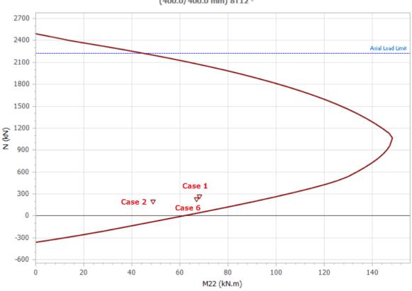
INTERACTION DIAGRAM (N-M) - 1C1N= 229.8 kN M22= 67 / M33= 0 kN.m (400.0/400.0 mm) 8T12 -
